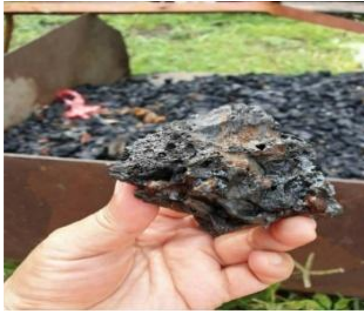
Figure 3: The result of burning plastic or foam boxes will turn into black lumps.
